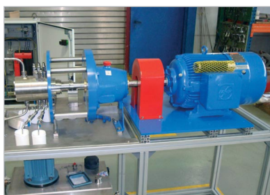
EDI Test rig for Pump packing.
